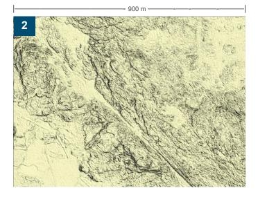
This novel Residual Elevation Attribute process can be employed in surface geologic studies for mining, oil, and geotechnical projects as it highlights any weak occurrence in the topographic relief. It can also be employed to study subtle man-made changes in topography.
