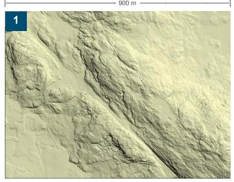
In **Figure 1**, a terrain model (in "shaded relief" mode) of a sample topographic surface was created from LiDAR data for an area in Canada.
